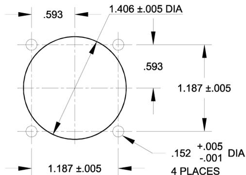
SUGGESTED MOUNTING HOLE LAYOUT FOR MOUNTING STUD
